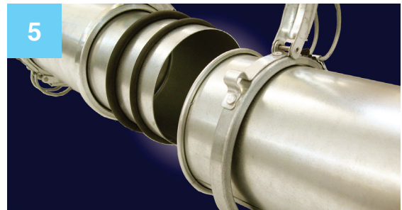
Place Slip Duct O-ring on the cut duct, then add the Oil Mist O-ring (which has a smaller thickness), and slide a Slip Duct over the cut end. Seat the Oil Mist O-ring evenly and firmly against the rolled metal edge of the Slip Duct. Then position the Slip Duct O-ring firmly against the Oil Mist O-ring.
